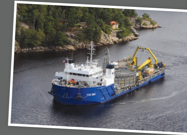
Cable installation vessel Team Oman was a wind farm stalwart. In total more than 100 kilometres of cables were installed offshore between the turbines and the offshore substations and from there to shore.
